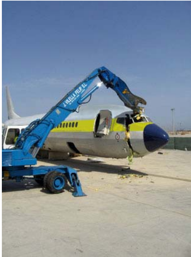
Shears are used to cut aircraft into pieces that the shredder can handle. It's a surprisingly simple process (Photos: AELS)
