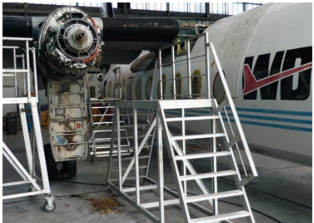
The first stage of a typical, sustainable end-of-life aircraft process is disassembly, whereby all valuable parts and components are removed from the aircraft for re-use.
